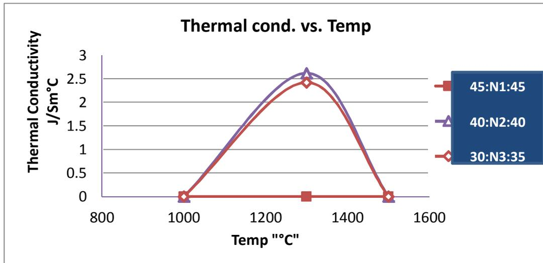
**Figure 3: Thermal conductivity versus Firing Temperature**
