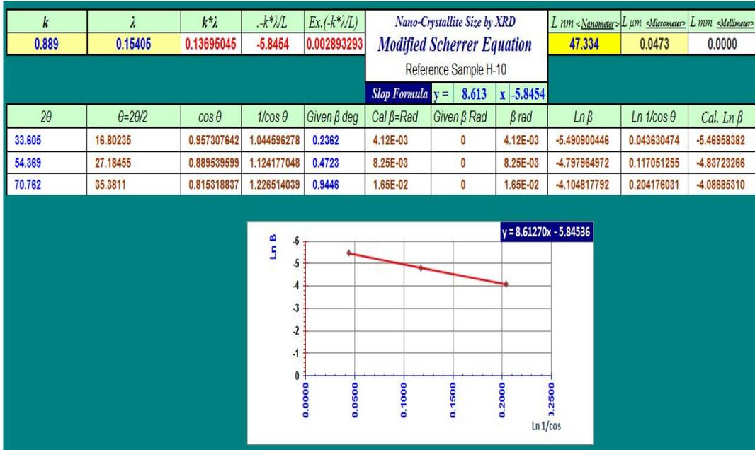
Figure 2: Computer calculation of crystallite size of nano – sized powder
