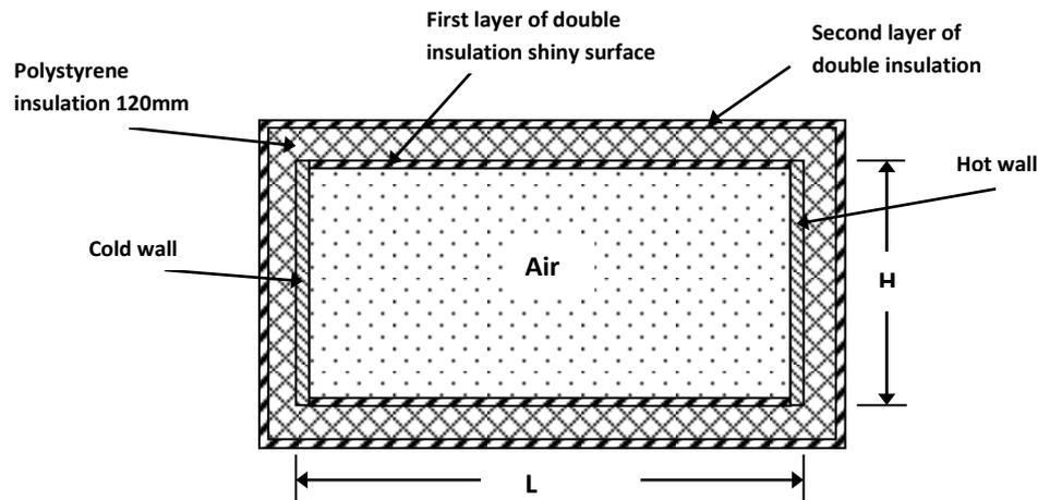
Figure 1 Schematic diagram of the enclosure with the hot and cold sides and all the insulation layers.
