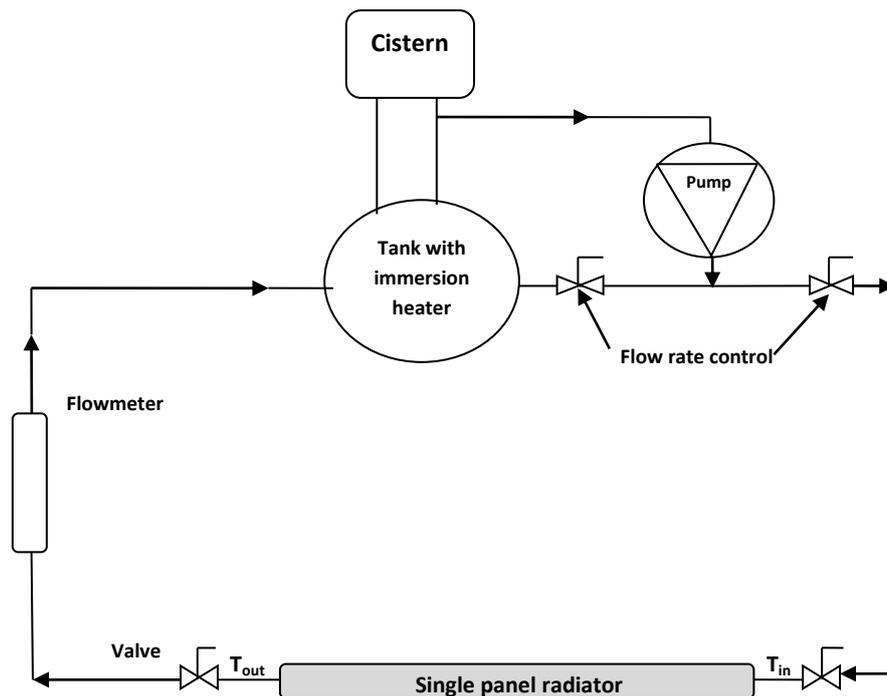
**Figure 2 Schematic diagram of the radiator hot water side.**
