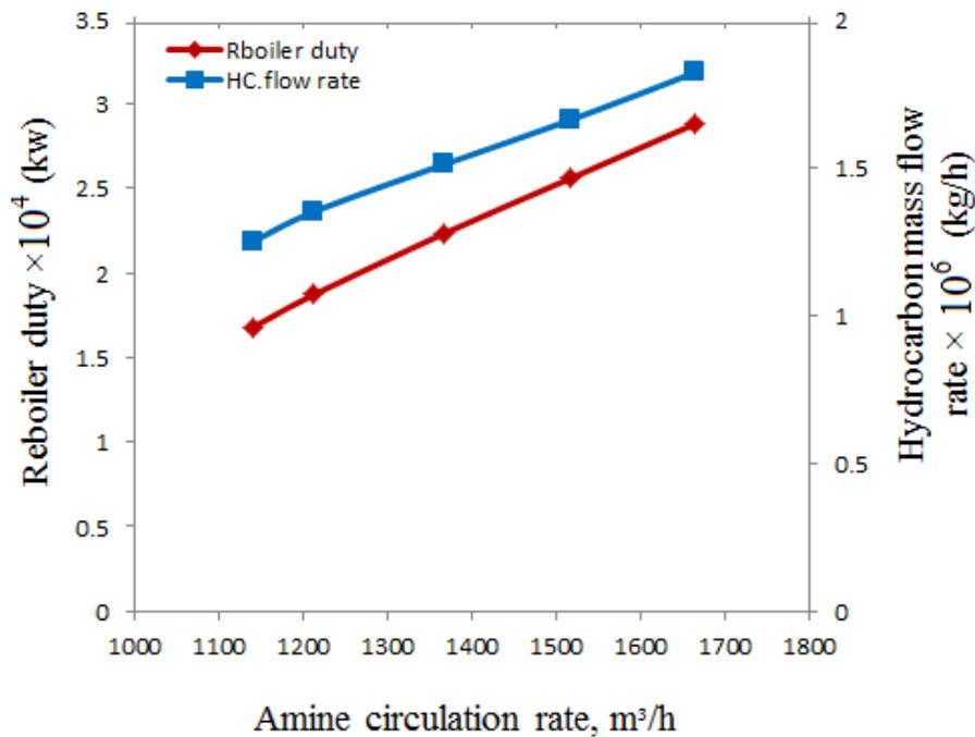
**Figure 8. Effect of MDEA & DEA blend circulation rates on hydrocarbons mass flowrate in the rich amine stream and reboiler duty**
