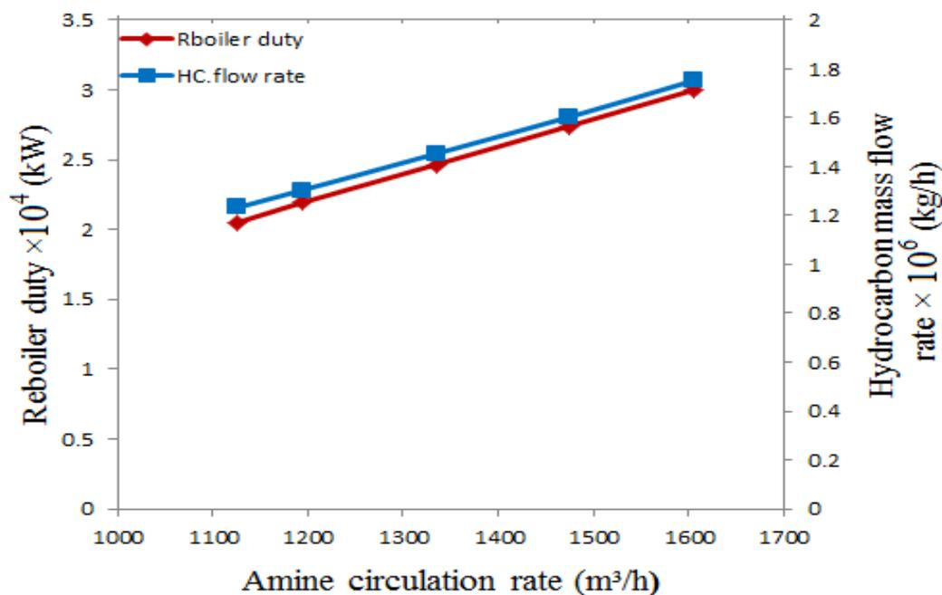
**Figure 9. Effect of MDEA&MEA blend circulation rates on hydrocarbons mass flow rate in the rich amine stream and reboiler duty required**
