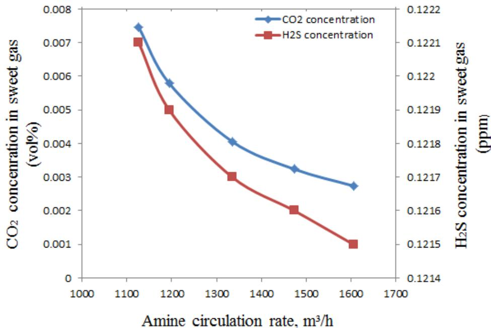
**Figure 7. Effect of MDEA & MEA blend circulation rates on acid gases concentration in the sweet gas stream**
