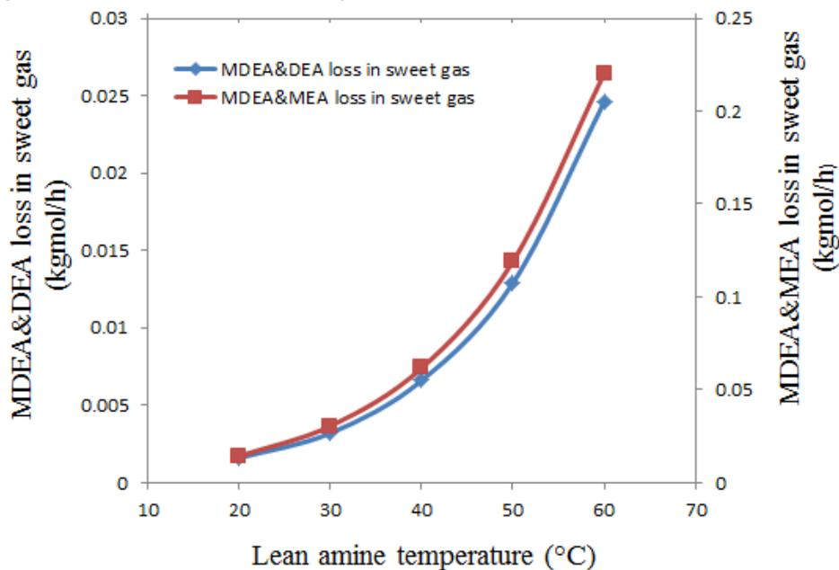
**Figure 10. Effect of lean amine temperatures on the losses of amines in the sweet gas stream**
