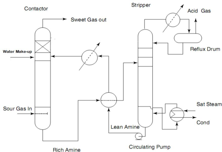
Figure 1: Typical gas sweetening process diagram
