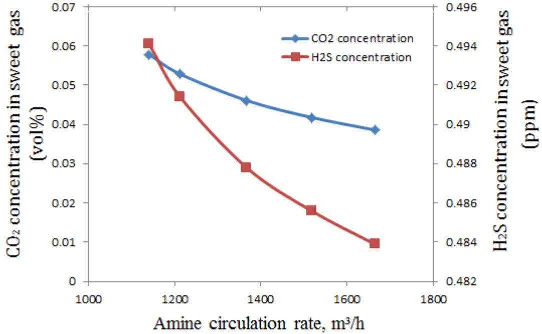
Figure 6. Effect of MDEA & DEA blend circulation rates on acid gases concentration in the sweet gas stream
