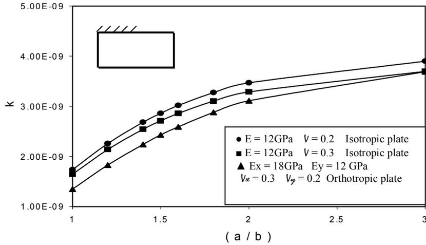
Fig. 6. Ratio of plate dimensions Vs. deflection factors at center of isotropic and orthotropic plate under uniform distributed load of 10 kPa.
