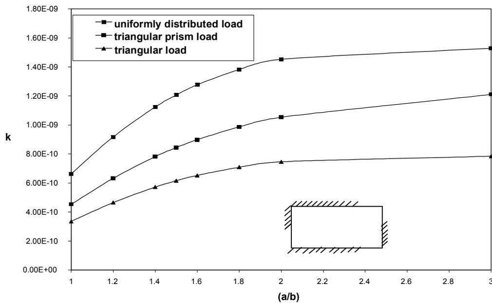
Fig. 4. Ratio of plate dimensions Vs. deflection factors at center of orthotropic plate for different types of load.
