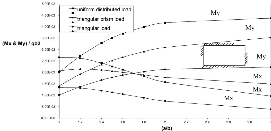
Fig. 5. Ratio of plate dimensions Vs. positive bending moments in x&y direction factors at center of orthotropic plate for different types of load.
