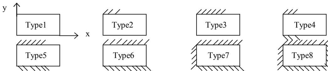
**Fig. 8.Orthotropic plates with different line boundary conditions subjected to equal uniform loading.**
