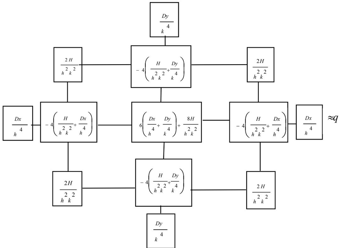
Fig. 1. Coefficient patterns of rectangular mesh for orthotropic plate [1].
