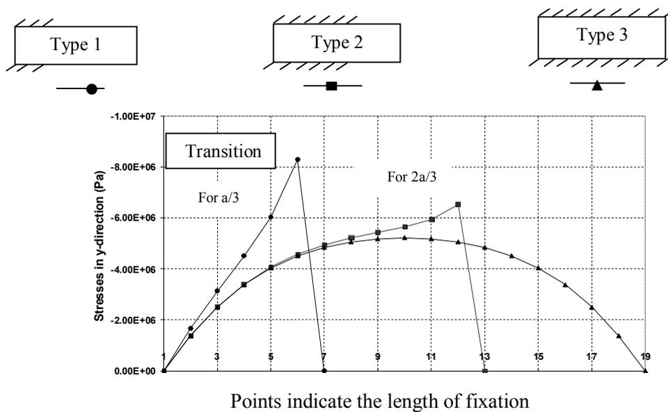
Fig. 9. Variation in stresses with increase in the length of fixation along the edge of orthotropic plates grid spacing (18 x 18).
