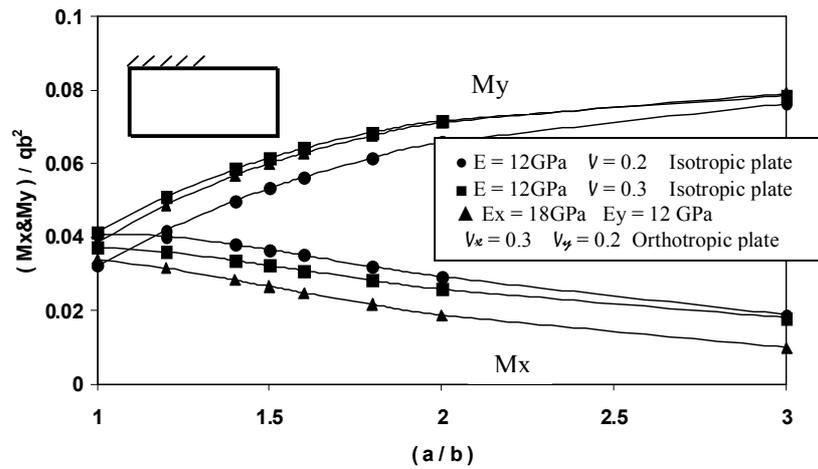
Fig. 7. Ratio of plate dimensions Vs. bending moment factors in x & y direction at center of isotropic and orthotropic plate under uniform distributed load of 10 kPa.
