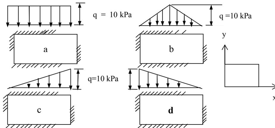
**Fig. 3. Cases of loadings of a selected orthotropic plate (2a/3 edge fixed + a/3 edge simply supported )**
